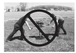
• Operators leaning too far over machine. Operator positions will not allow for proper reaction and control in the event of kickback.
