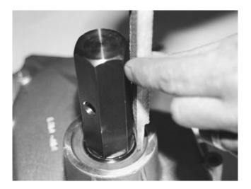
15) Reinstall the upper bearing cone, Nilos ring and Woodruff key on the final driveshaft. Coat the Woodruff key area of the driveshaft with light oil or with the Barium or Lithium based lubricant. Reinstall the secondary gear and flat washer.
